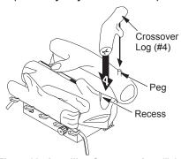
Figure 32 - Installing Crossover Log (#4) (Base may very from illustration)
